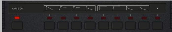
*Vari 2 showing the Envelopes used for the Saxophone preset. No envelopes from the menu are selected, indicating that the Saxophone preset uses one of the “hidden” envelope setting for each envelope group.*
