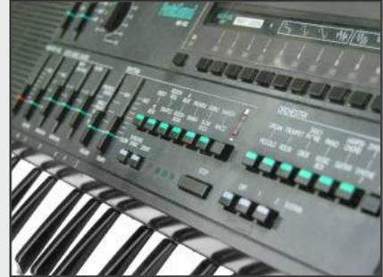
The in-built sequencer was crude - you could record a song of chords for the auto-accompaniment section, and separately a monophonic line over the top, alongside your custom drum and bass patterns, and you could save the entire state of the instrument to a cassette interface - common on more pro-gear at the time, but not seen on domestic portable keyboards.
