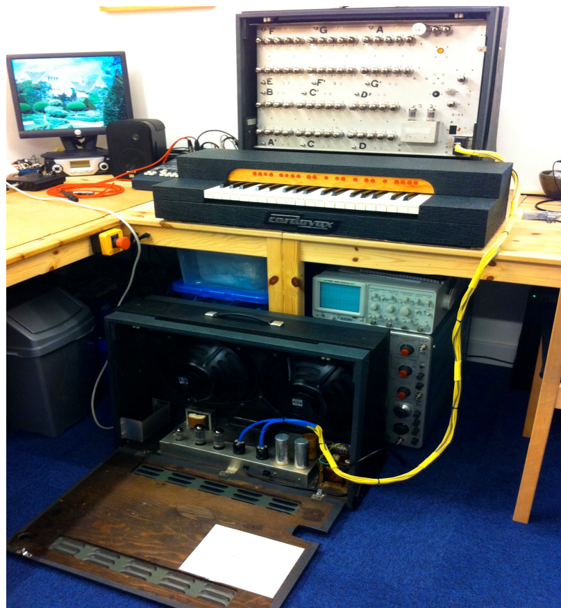
The bizarre custom Cordovox CG-1 tube polysynth I originally built for Will Gregory
